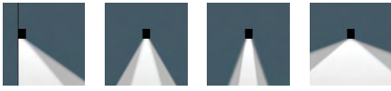
[R45] Rectangular 'side throw' [M] Symmetric, medium beam [E] Symmetric, narrow beam [S] Asymmetric 'side throw'
