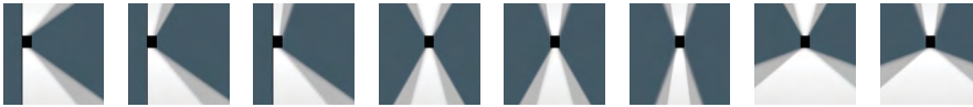
[R45/R45] 'Side throw', up and down [M/R45] Medium beam up, 'side throw' down [E/R45] Narrow beam up, 'side throw' down [M/M] Medium beam, up and down [E/M] Narrow beam up, medium beam down [E/E] Narrow beam, up and down [M/S] Medium beam up, 'side throw' down [E/S] Narrow beam up, 'side throw' down
