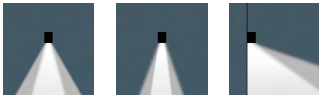
[M] Symmetric, medium beam [E] Symmetric, narrow beam [A60] Asymmetric 'forward throw'
