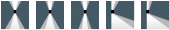
[M/M] Medium beam, up and down [E/M] Narrow beam up, medium beam down [E/E] Narrow beam, up and down [M/A60] Medium beam up, 'forward throw' down [E/A60] Narrow beam up, 'forward throw' down
