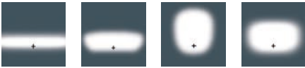
[P65] Pedestrian / bicycle lane [S65] Streetlighting [A60] Asymmetric 'forward throw' [R65] Rectangular 'side throw'
