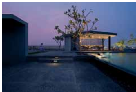
03 Steplights facilitate orientation by marking paths, or by reducing the risk of tripping up by illuminating different levels on platforms and terraces.
