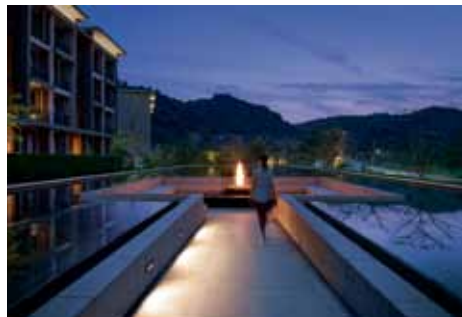
02 Often used where gentle glare-free lighting and well-placed accents are required, recessed luminaires near ground level can be used to create atmosphere even at low wattages.
