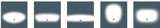
[S60] [S65] [S70] Streetlighting [A60] Asymmetric 'forward throw' [R65] Rectangular 'side throw'
