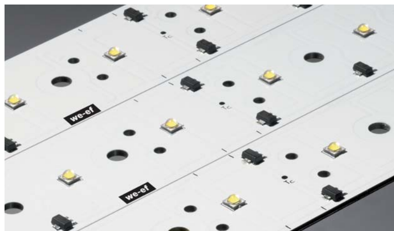
WE-EF LED boards fitted with high-quality LEDs, which have narrowly-defined binning tolerances, guarantee high-visual comfort.
